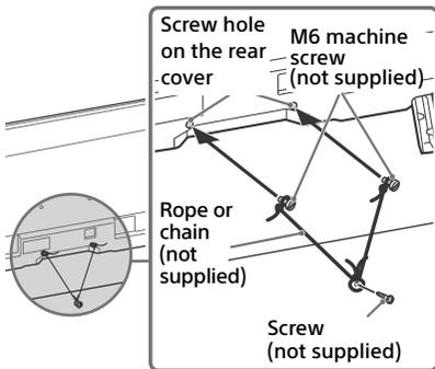
The length of the M6 machine screw differs depending on the rope or chain diameter. Please refer to below illustration.
