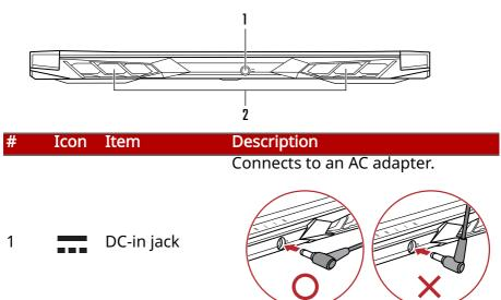
Note: Please press the AC adapter into the tunnel to the power connector. You will feel a click indicating it is connected. Then, check the light of battery indicator shows amber while charging.
