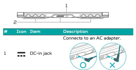
Note: Please press the AC adapter into the tunnel to the power connector. You will feel a click indicating it is connected. Then, check the light of battery indicator shows amber while charging.
