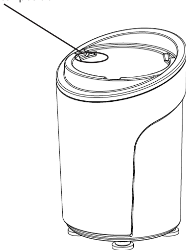
Safety switch position
