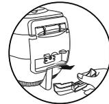
After cooking or warming, throw the water out of dew dish. Failure to remove contents in the dew dish will cause an odor to appear.
