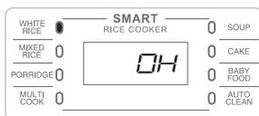
"0H" on the display panel means that the cooked rice has been kept warm for 0 hours.
