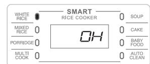
When reheating is done, the Keep Warm function will start again, and the amount of time that the Keep Warm mode has been functioning will be displayed.
