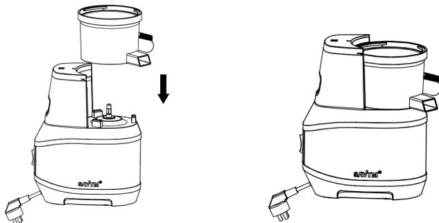
2. Install filter components (the triangle mark on the filter must be aligned with the one on the juice container)
