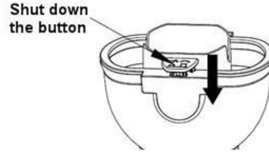
9. Press Button "ON/OFF" when food is processed and no more juice flow out. After the motor and screw stop completely, take the juice cup away from juice mouth and slag door
