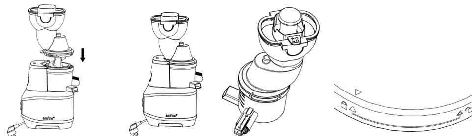
5. Put cup on the both sides of juice mouth and slag door, put pusher on.
