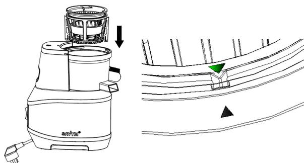
Arrow is at the top of the filter holder, the arrow is relatively small, look for it carefully.
