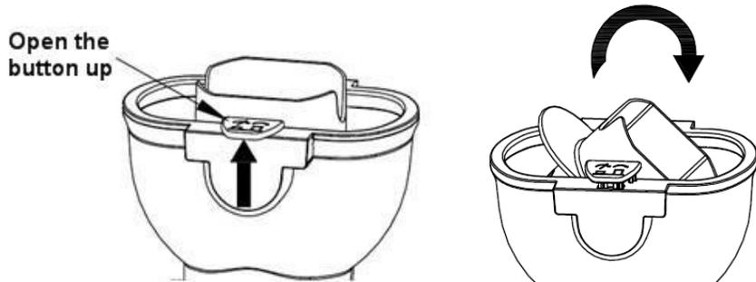
·Shut down the button, and lock swivel bracket when squeeze small volume of fruits such as tomatoes, small orange, peeled pomegranate etc., then put the ingredients into feed inlet.
