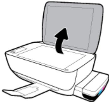
2. Load the original print-side down on the right corner of the scanner glass.
