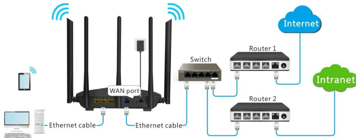
Connect Router 1 to the internet and Router 2 to the intranet. AC7 gets IP address to access the internet from Router 1 automatically. To make both the internet and the intranet be accessible to devices on the LAN network, set static router on AC7.
