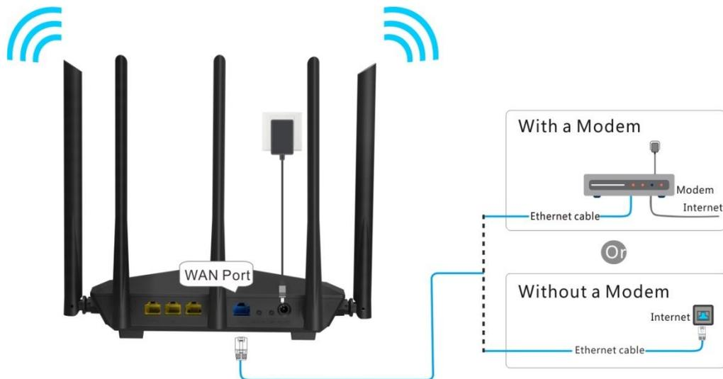
4. Connect your computer to port 1, 2 or 3/IPTV of the new router using an Ethernet cable.
