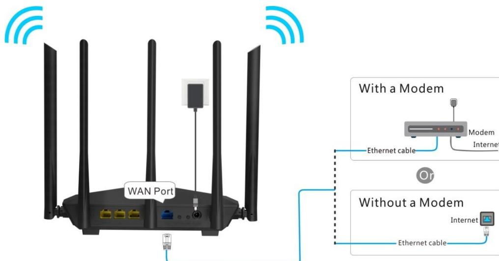
4. Connect your computer to port 1, 2 or 3/IPTV of the router using an Ethernet cable.
