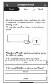
② Check that the Wireless LAN LED is ON. Press the Wireless LAN ♠ button for 5 seconds until "1" appears on the remote control. Point the remote control to the air conditioner and press SET.
