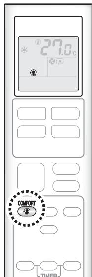
The flow of air will be in the upward direction while in COOL operation, which will provide a comfortable wind that will not come in direct contact with people.
