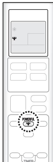
POWERFUL operation quickly maximizes the cooling effect in any operation mode. You can get the maximum capacity.
