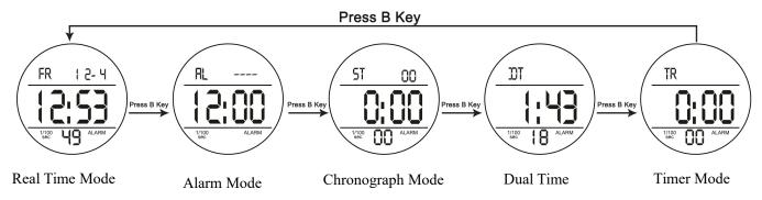
At any state ,press A or E key EL backlight for 2s.
