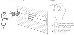
Leave a 0.4 inch (9 mm) gap between the wall and the screw's head. Lift the soundbar over the heads of the screws and slot into place.
